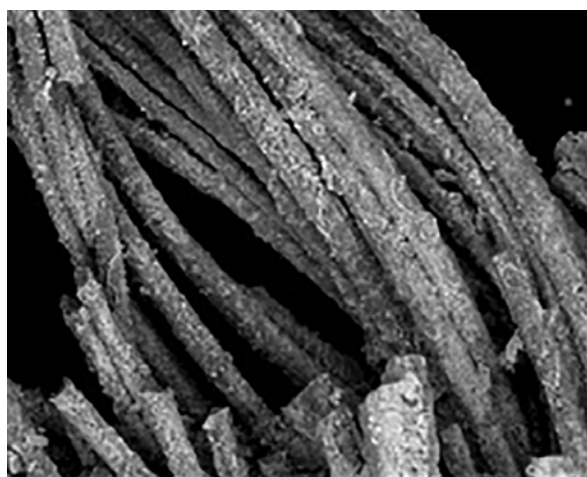
Figure 6.30: Scanning electron microscope image of individual wool fibres. Image: Lore Troalen and Susanna Harris.
