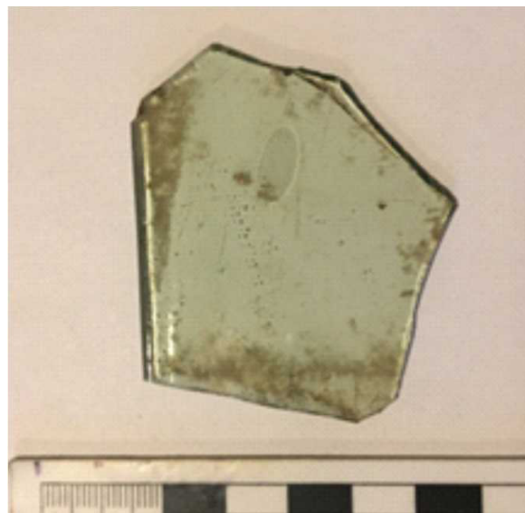
Plate 98: A piece of Type 2 glass showing the smooth straight edge (LHS) and a large elongated air bubble characteristic of the cylinder method of manufacture
